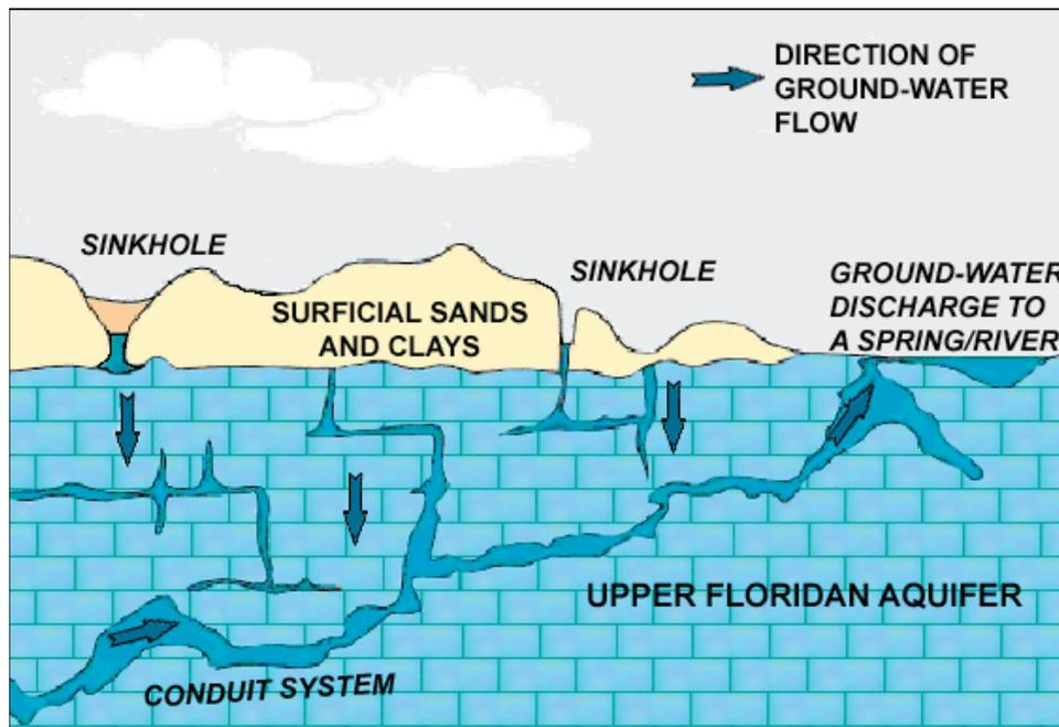
*Figure 1: Geologic cross-section showing entry points to groundwater contamination. Source: USGS. The Suwannee River Basin Pilot Study.*
