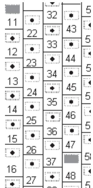
Figure 4—Illustration by author of a section of a punch card ballot. When a vote is recorded, the perforated rectangle (with a dot) is punched out of the card (as shown for areas # 11 and #48). There is no indication for voters on the ballot regarding which punched hole corresponds to which candidate.
