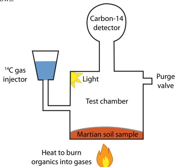
Figure 3. Set-up of PR experiment.
