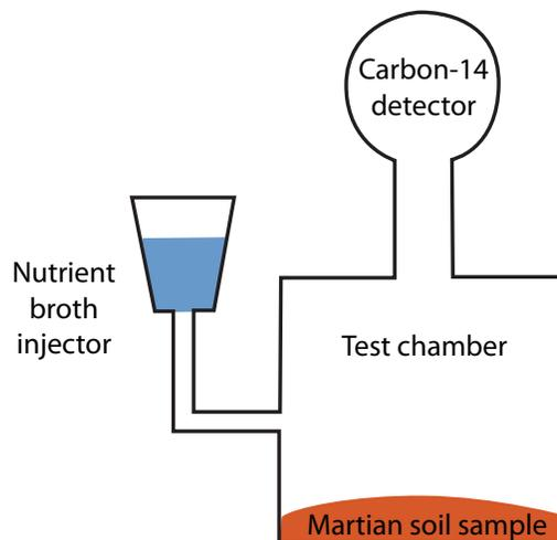
Figure 1. Set-up of LR experiment.
