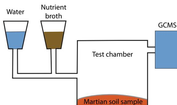
Figure 5. Set-up of GEx experiment.
