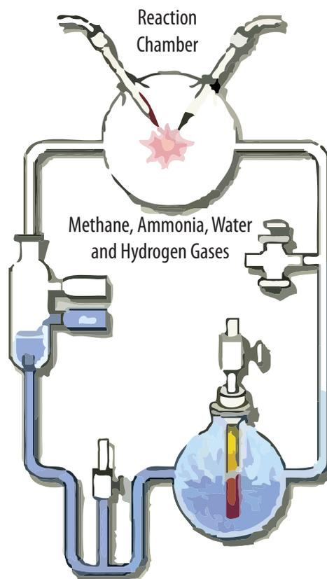
Figure 1. Stanley Miller's experimental set-up.
